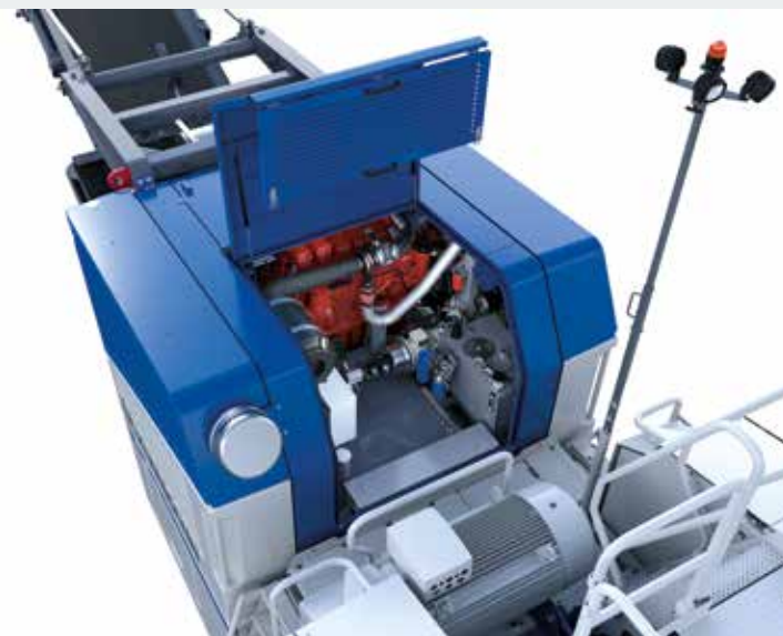
> MC 120(i) PRO - easiest possible access to the engine compartment
