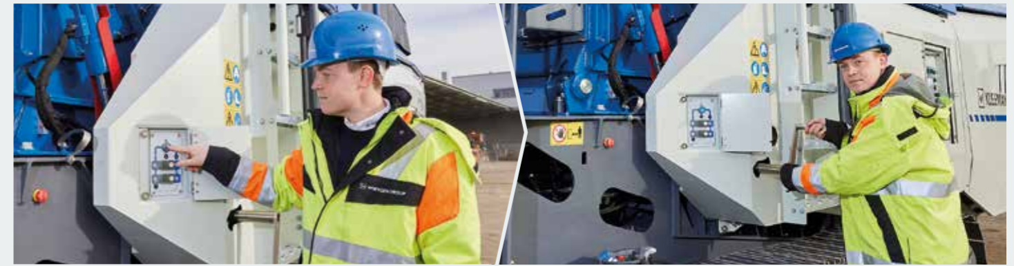
> The rotor locking and turning device is released at the touch of a button... ...and engaged by hand crank.
