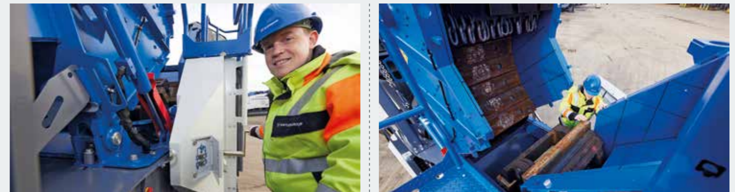
> The rotor is moved into position for wear check or rotor ledge replacement. > The crusher is opened completely for best possible access for service and maintenance from both sides. Rotor ledge replacement takes place easily from above.
