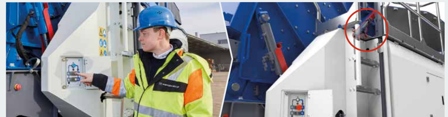
> The crusher is unlocked at the push of a button... ...and the wedges for locking the crusher housing are pulled hydraulically.
