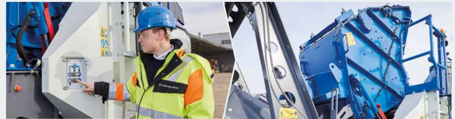
> Automatic opening of the crusher housing when the button is held down... ...until the crusher opens completely. The mechanical safety catch also engages.
