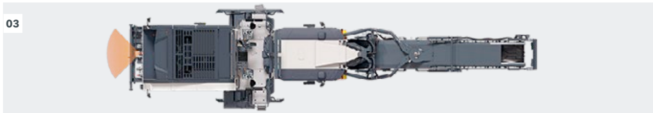
Standard camera system comprising one camera: area in front of the machine
