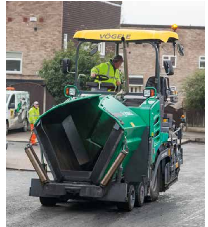
The push-rollers automatically fold up together with the hopper sides.
