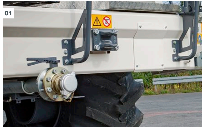
01 The hose connection is mounted on the front crossbeam.
