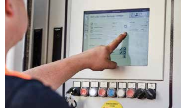
> Trigger the "Lock rotor" command via SPECTIVE
