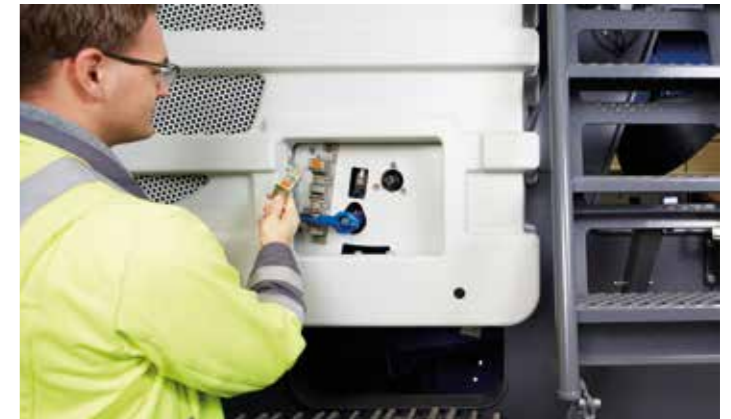
> If keys are removed, the rotor remains safely locked.
