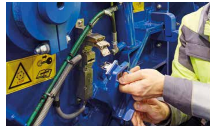
> The crusher housing is opened with a special key. The key cannot be removed once opened and material can be cleared safely.
