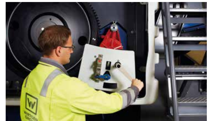
> The rotor is turned safely with the crank and moved into the optimum position for rotor ledge replacement.
