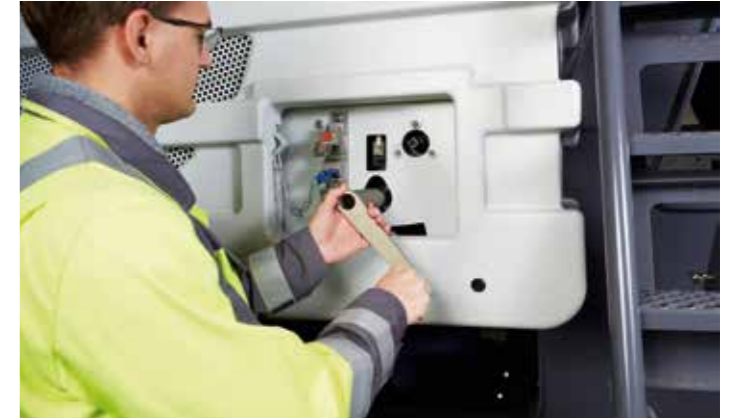
> The rotor locking and turning device is enabled and can be moved with a crank.
