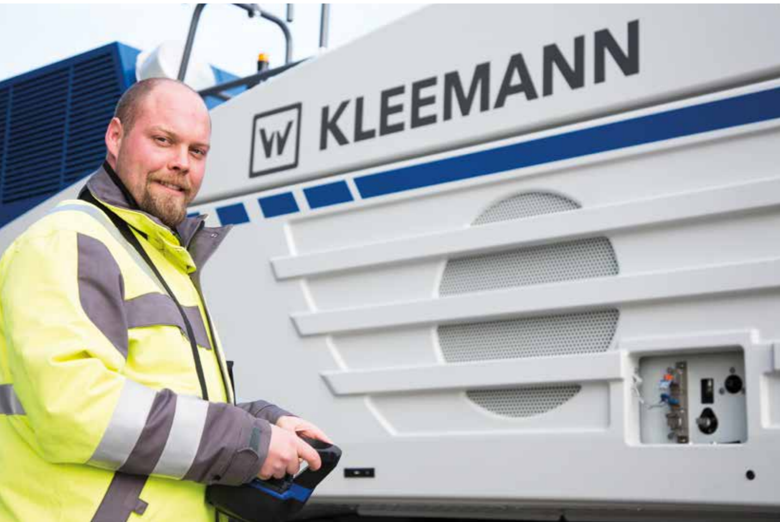
> Insert control element in the enable station; the rotor is safely locked and the key is enabled for further steps.
