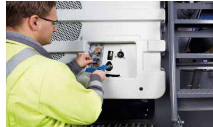
> Insert control element in the enable station; the rotor is safely locked and the key is enabled for further steps.
