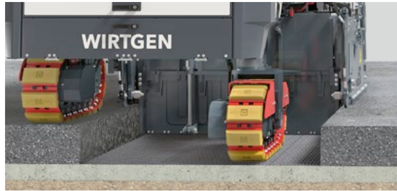
Milling drum assembly FB1800 with Multiple Cutting System MCS BASIC .
