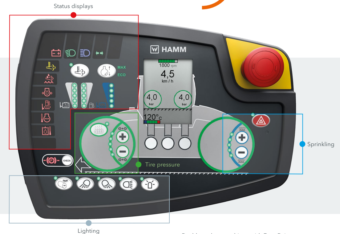
Dashboard on machines with Easy Drive (EPA Tier 4/EU Stage V)
