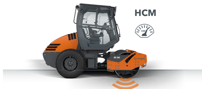
Thanks to their even weight distribution, the compactors have high traction, even on rough terrain.
