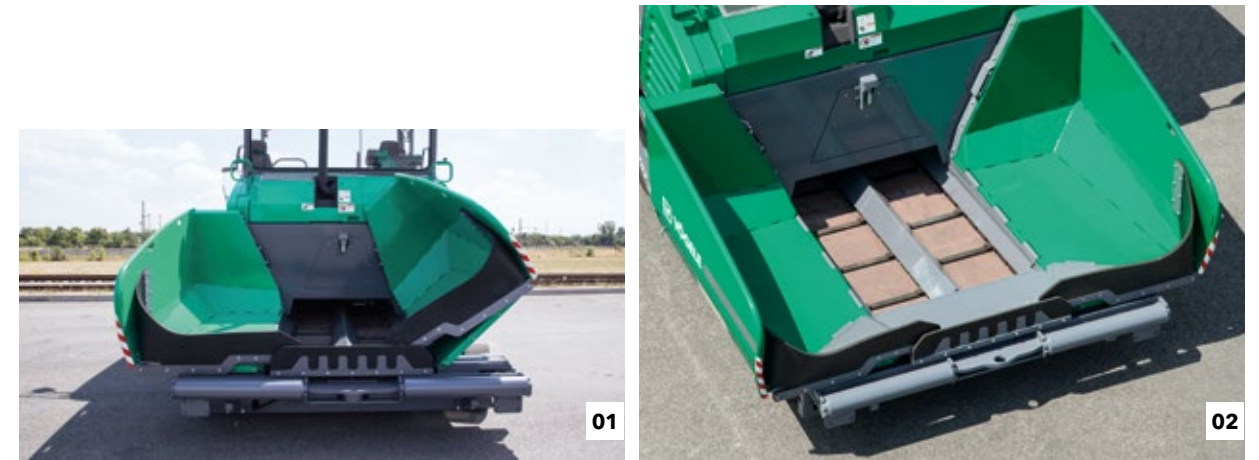
01 Independently operated hopper wings. 02 The large material hopper holds 14.3 tons (13 tonnes).
