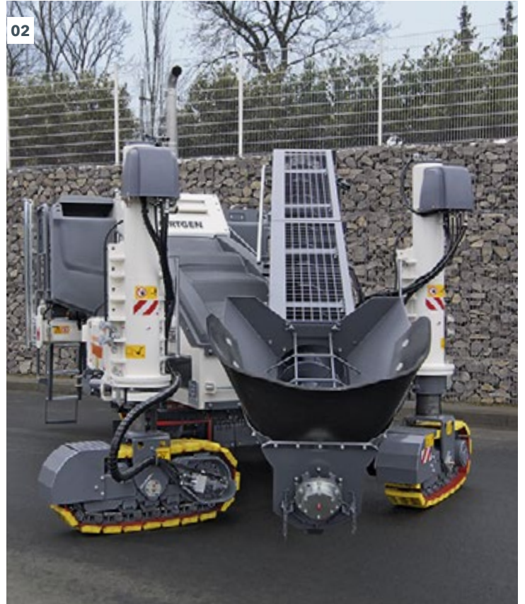
01 - 02 The SP 15 i can be equipped with either a belt or an auger conveyor.
