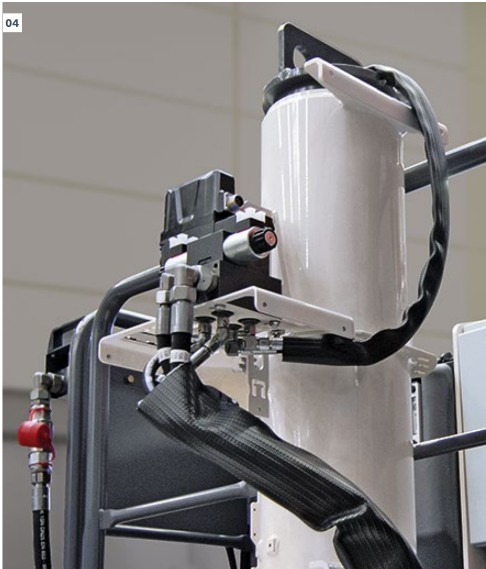
01 Software developed in-house guarantees maximum operational safety. 02 - 03 The high-quality machine control system ensures that the machine can travel both perfectly straight and precisely around curves. 04 Separate valves on all crawler units for high-precision control of height adjustment and steering.
