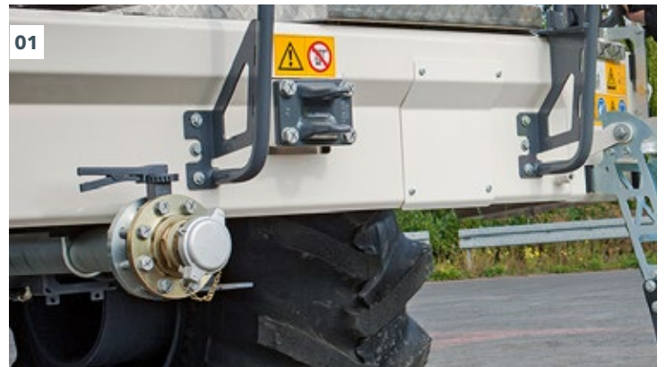
01 All of the hose connections are attached to the front cross member.
