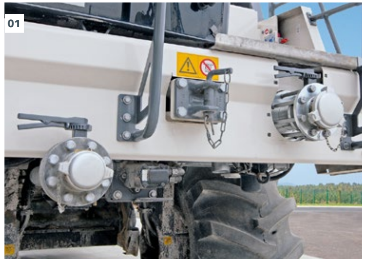
01 The filling connector for foamed bitumen is easily accessible.
