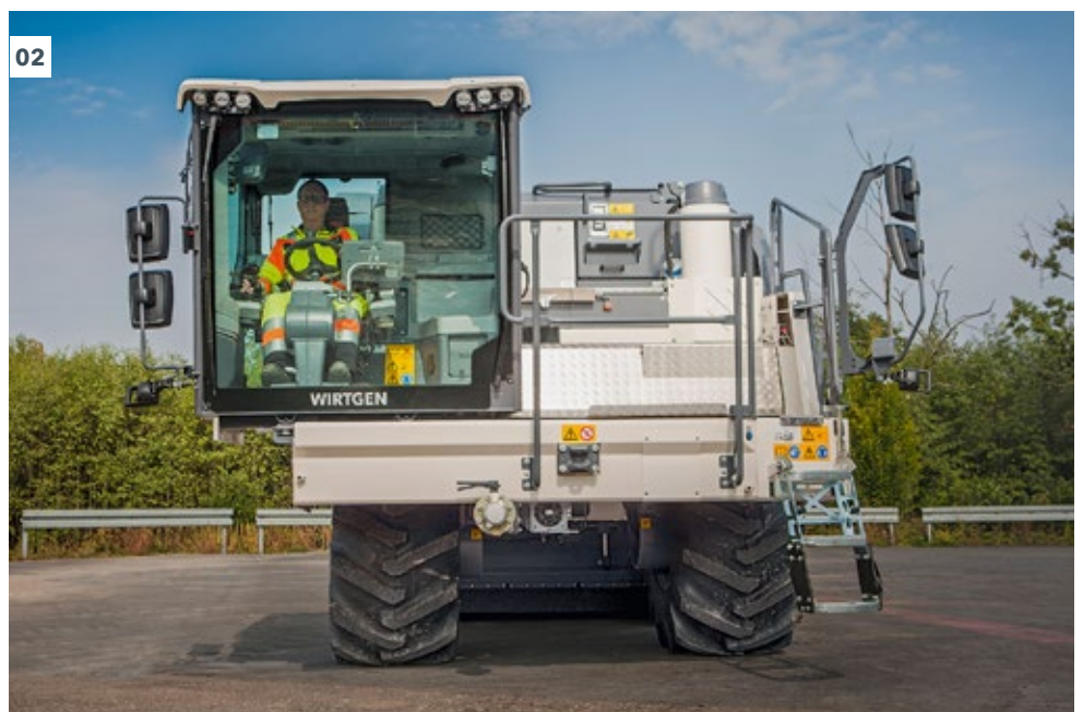
01 - 02 The operator's cabin can be moved far to the right hydraulically, allowing the operator to look past a recycling train traveling ahead.
