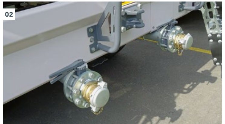
02 Connections for water and emulsion are easily accessible.
