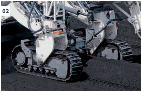
02 - 03 All four track units can be adjusted in height separately via hydraulic cylinders.
