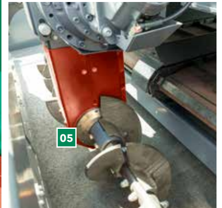
Components particularly protected by the Heavy-Duty kit (shown in red): 01 Scraper for the hopper sides 02 Lateral guards of the conveyor chains 03 Central guard of the conveyor chains 04 Conveyor tunnel 05 Centre auger bearing box
