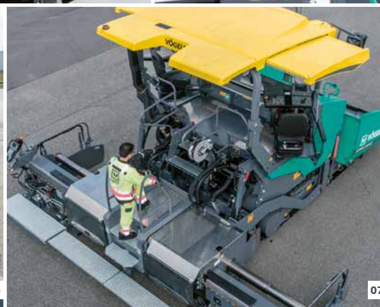
05 PaveDock Assistant simplifies communication during transfer of material. 06 Well-organised, ergonomic workstation. 07 Safe, convenient step onto screed.
