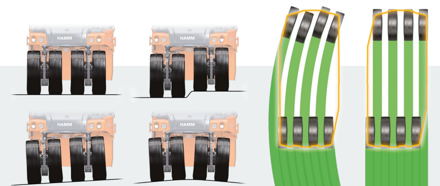
The generous overlapping of the tyre tracks contributes to complete and even compaction.
