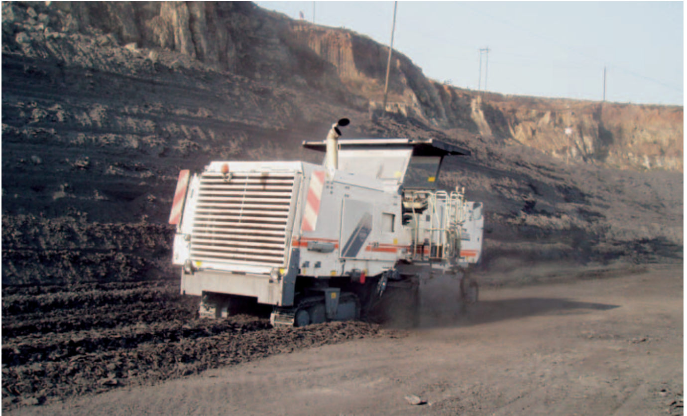
The Surface Miners ensure the selective extraction of the coal deposits. Indian coal has a high inherent ash content. Selective mining guarantees high quality coal for the energy industry.
