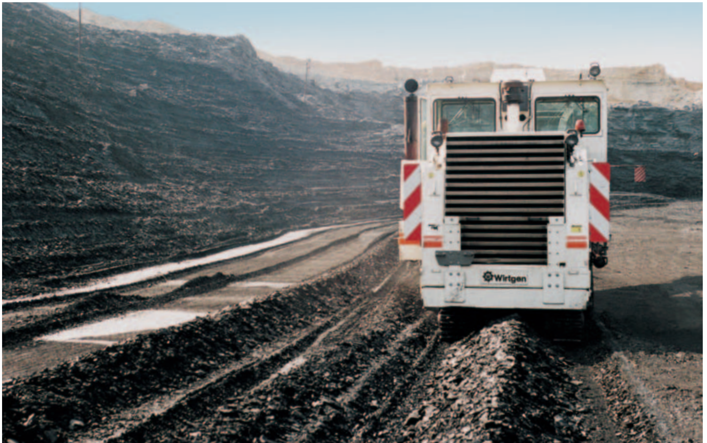
The coal can be cut and crushed in one machine pass with low manpower requirements. The material is deposited in a windrow behind the machine, ready to be loaded.
