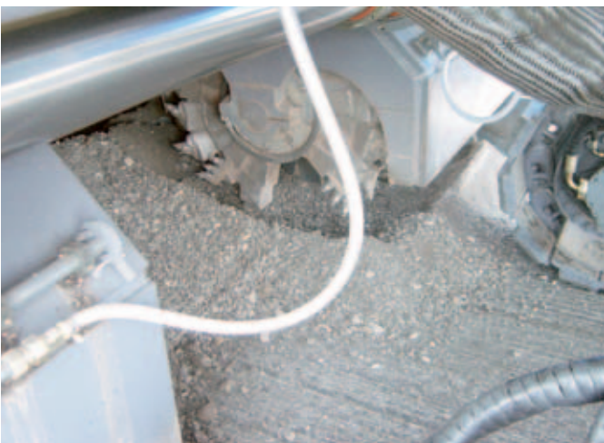
View of extendable down cutter.
