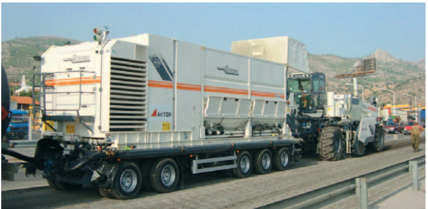
The Wirtgen WM 1000 cement slurry mixing unit manufactures up to 1000 litres of cement slurry per minute, drawing from on-board storage facilities. The amount of water added is adjusted to meet the moisture demands of the recycled material. The slurry is pumped to the recycler where it is injected into the milling chamber under pressure through a spraybar separate from the one used to foam bitumen, thereby ensuring the best mix quality possible.
