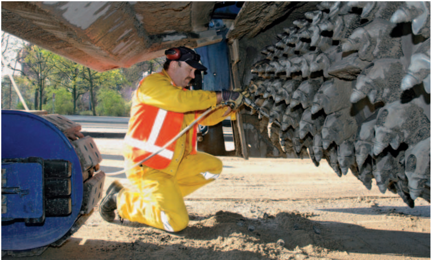
Their improved rotation gave Betek's new cutting tools of the R-series a significantly higher durability when compared to conventional tools, even when working in hard concrete.
