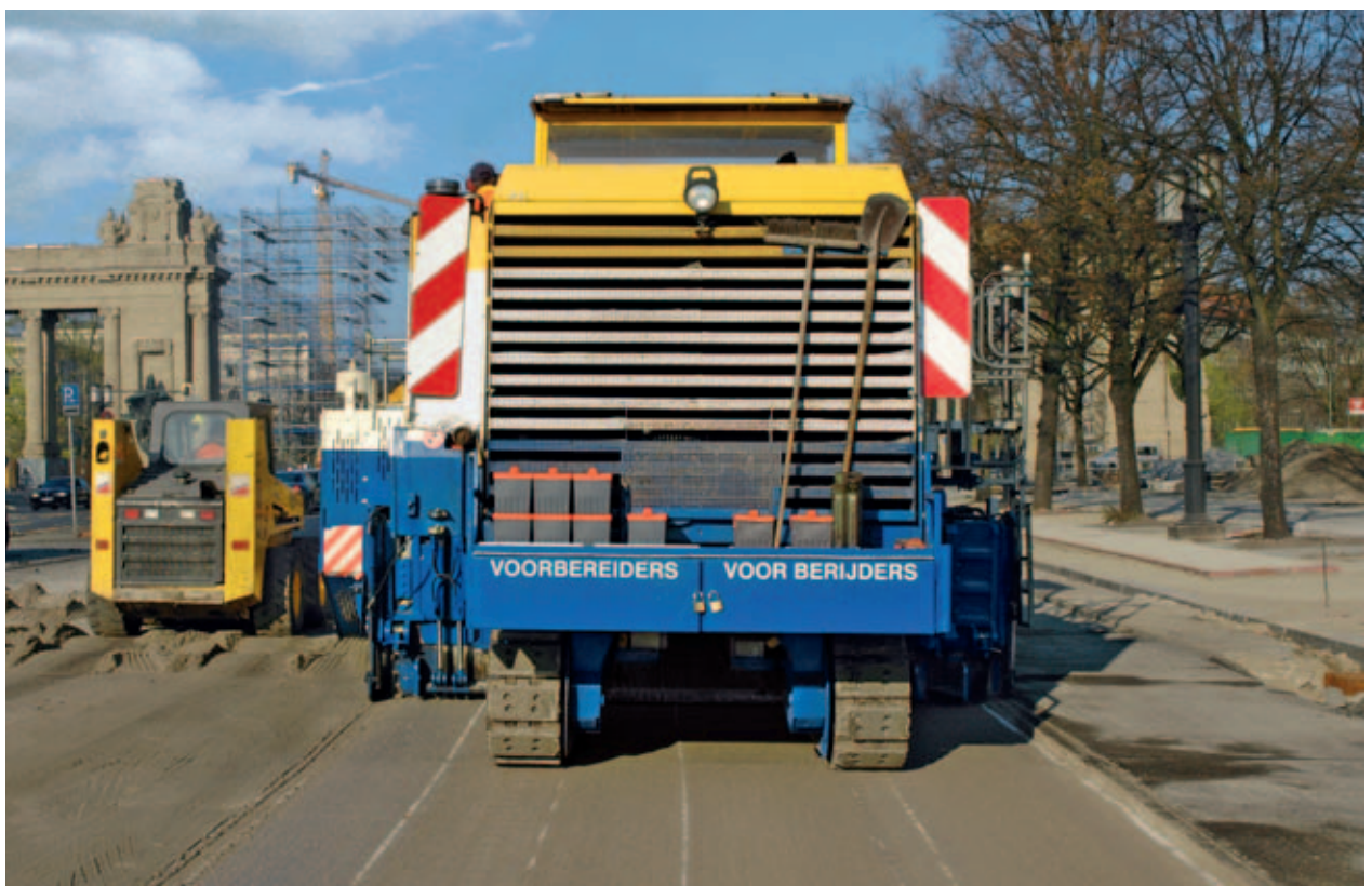
With an engine output of 671 kW (900 HP), the Wirtgen W 2200 has ample power reserves that enable it to mill pavements at depths of up to 35 cm or hard concrete pavements at large advance speeds even when working with the 3.80 m wide FCS drum unit.
