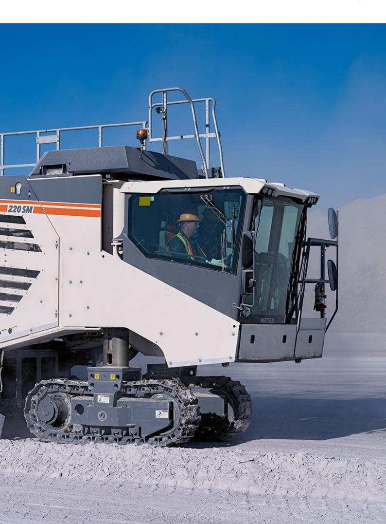
The 220 SM(i) is the prime choice not only for use in small and medium-scale mining operations but also for routing work and infrastructure projects. The compact, multipurpose surface miner extracts primary resources with an unconfined compressive strength of up to 50 MPa selectively and at a cutting depth of up to 350 mm. The 2.2-m wide cutting drum unit is tailored precisely to the specific application and guarantees high productivity at low operating costs.
