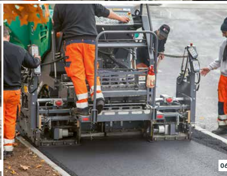
05 Fully integrated Niveltronic Basic system for automated grade and slope control. 06 Can be combined with the AB 200 V and AB 220 V extending screeds.
